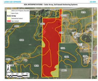
Figure 13: Soil Interpretations for Solar Arrays, Soil-based Anchoring Systems
